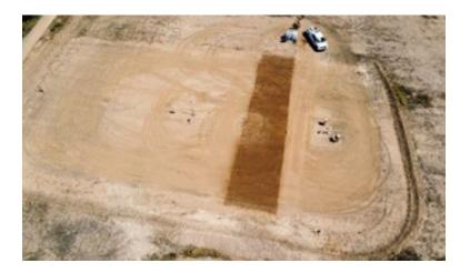
FIGURE 43 Aerial view of EICP treatment at the Salt River Landfill.
