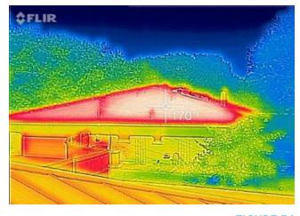
FIGURE 34 Attic heat underneath asphalt shingles. (Credit: <u>Green Building Advisor</u>)
