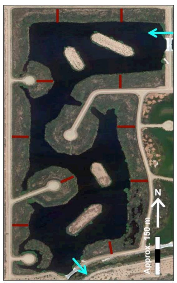
Figure 1. Constructed wetland study cell Arrows indicate location and direction of inflow(top arrow) and outflow(bottom arrow) sites. Red lines indicate transect locations.
