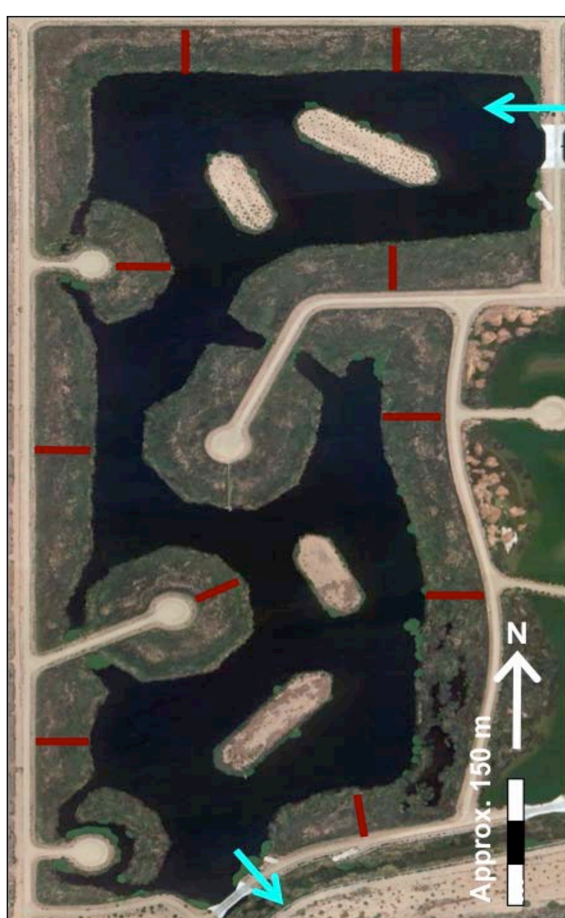
Figure 2. Constructed wetland study cell with approximate locations of 10 bimonthly sampled transects (denoted by red lines).
