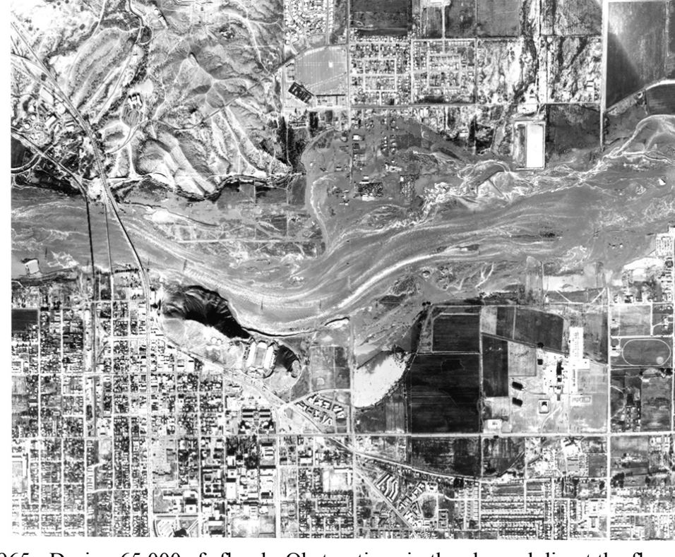
December 1965 - During 65,000 cfs flood - Obstructions in the channel direct the flow southward
