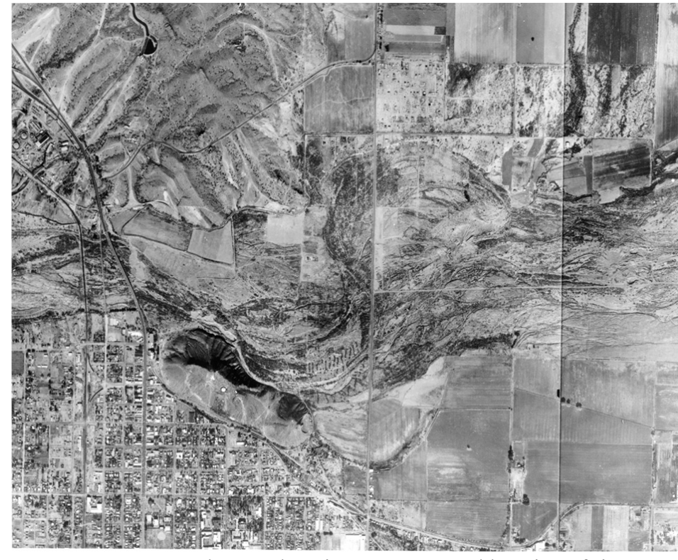
January 1954 - Encroachment changing geometry and location of river course
