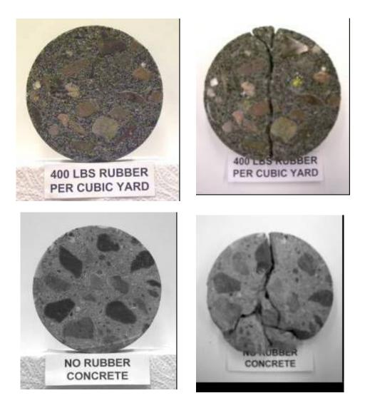
Figure 4 Tensile Strength Failure Mechanism.
