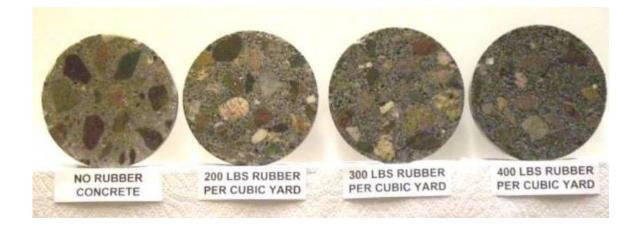
Figure 2 Cross Sectional View of Crumb Rubber Content Variation in Trial Mixes.
