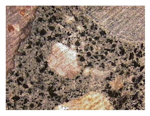
Figure 3 Microscopic View of Crumb Rubber Distribution in a 400 lbs CR / Cyd Mix.
