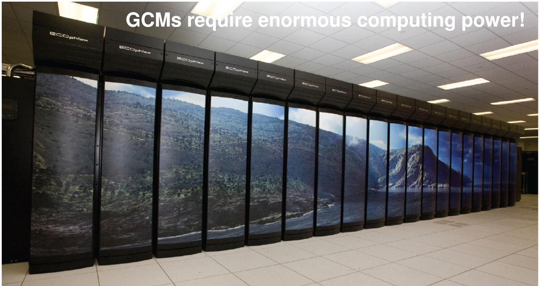
FIGURE 1.5 Global climate models are run on supercomputers, like the NOAA climate research super-computer Gaea at Oak Ridge National Laboratory in Tennessee (pictured). It has a peak speed of 1.1 petaflops (more than 1,000 trillion calculations per second). SOURCE: ORNL photos/Jay Nave (<http://blogs.knoxnews.com/munger/2011/12/noaas-petascale-computer-for-c.html>).
